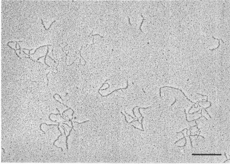
Figure 3. Electron micrographs of native xanthan sample E. The electron micrographs were obtained from replicas prepared as described in Figure 1. Scale bar = 200 nm.
